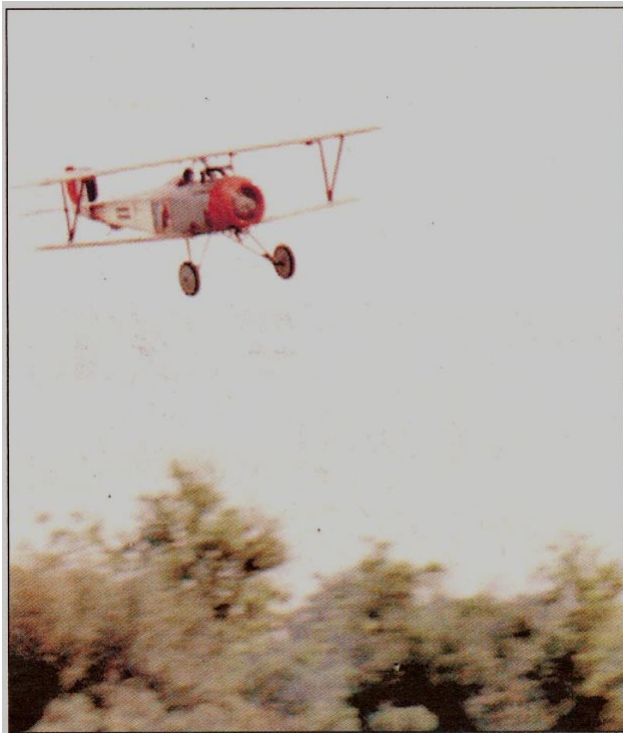
A World War I French Nieuport fighter comes in for a low pass. Giant scale aircraft like this one are often powered by converted chainsaw or gasoline weed trimmer engines.
