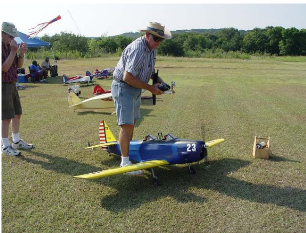
Roger Walther;s PT-19, Dynaflythe Kit w/a Super Tiger 3000, 88" WS and showing it in flight
