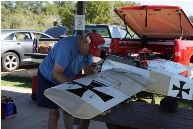
Hubert setting up wing support wires on the Eindecker
